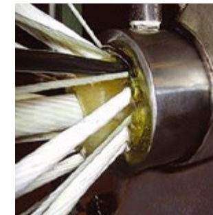
Filling all voids during cable manufacturing
