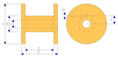
Habia Cable can deliver on a number of standard spool sizes provided that the inner diameter of the spool remains consistent with the cable's Minimum Bend Radius (MBR). For an simple guide, the dimension 'B' should be 20x the diameter of the cable (e.g. Spool SD100/60K has a inner diameter 'B' of 60mm. The maximum core size suitable for this drum would be 3mm).
